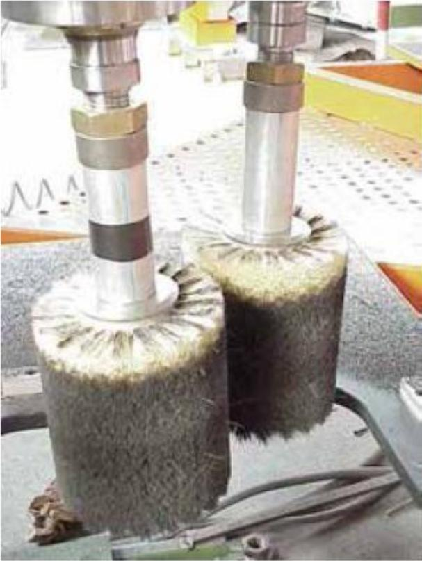
The working stations 233F-277F in the positions 3-4-6 are equipped with a single mandrel tool holder head on which a tool for the polishing of the bowl's bottom is installed (mushroom brush)
