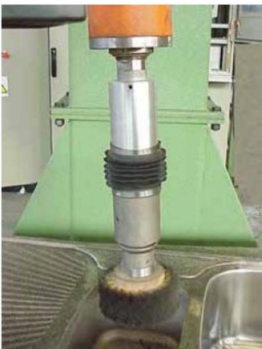
The working station 277P in the position 2 is equipped with a two-mandrel tool holder head on which both a tool for the polishing of the bowl's bottom (mushroom brush) and a tool for the polishing of the bowl's wall (cylindrical brush) are installed.
